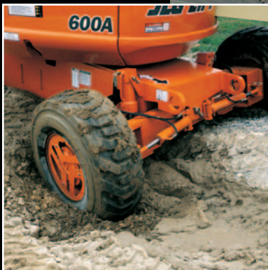
Oscillating Axle for Tough Terrain
