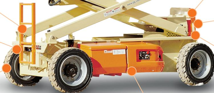
Tie down and lifting lugs for ease of transport
