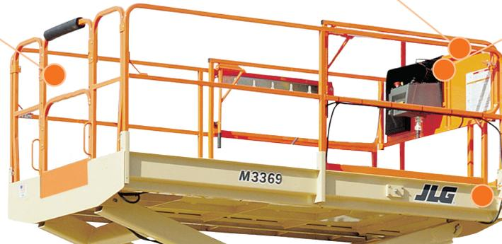
Low maintenance non-skid steel platform with extension deck and Load Sensing System
