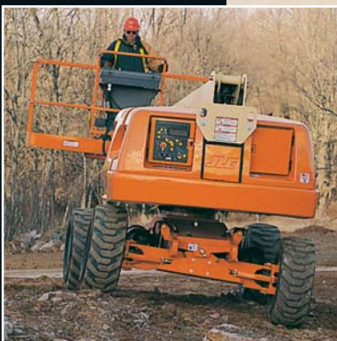
Oscillating Axle for Tough Travel
