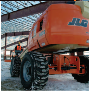
Oscillating Axle For Improved Traction & Drive Performance
